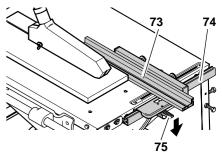
Danger! Always use the push stick if the distance between saw blade and rip fence is less than 120 mm.
